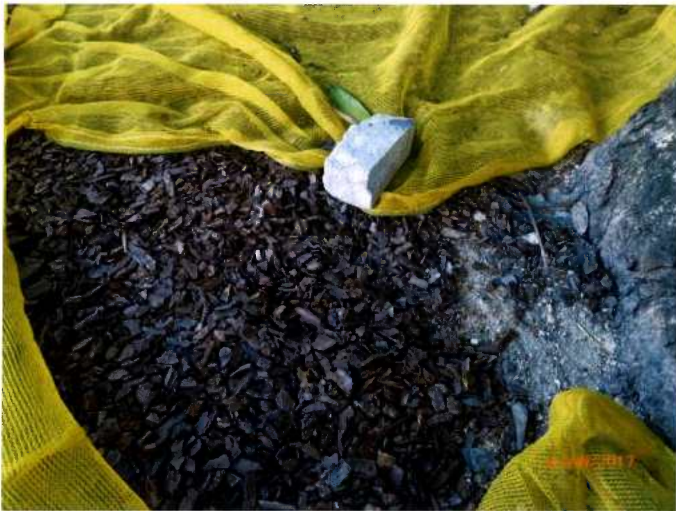
Fig. 11 Size of the mulch is too small, not up to ASD Spec. required standard.
